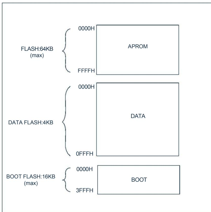
CMS8S589x can configure the size of BOOT, the configuration method is as follows:
