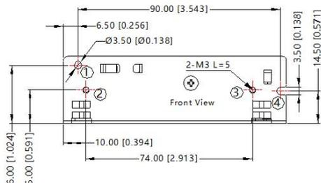
①-⑧ any position must be connected to the earth( )
