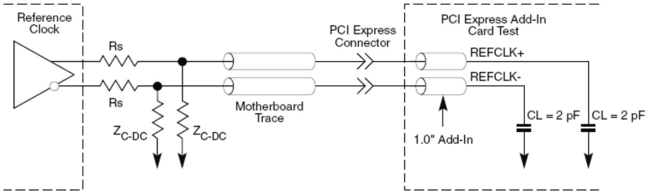
**Figure 12. Reference Clock System Measurement Point and Loading**
