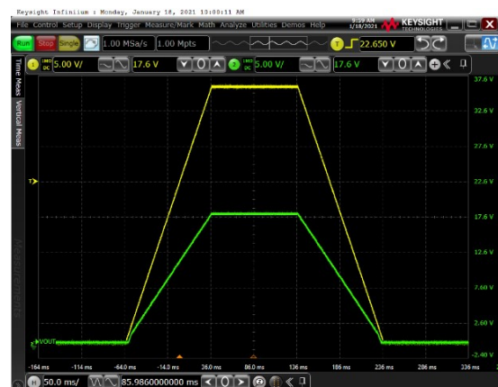
Figure 10. Power-on and Power-off Behavior, 2 ms
